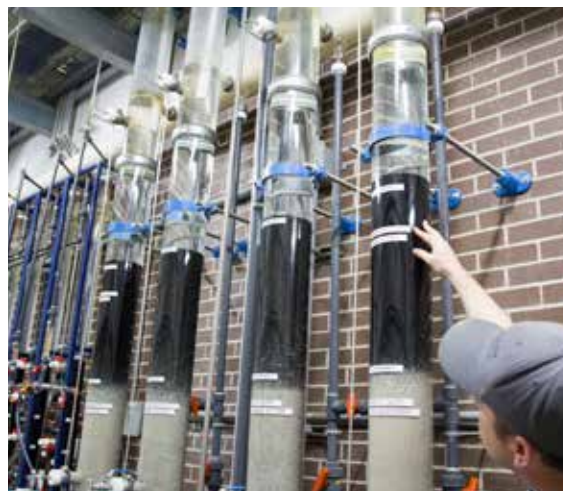
A coagulation study was completed, using an ozone contactor and biofiltration columns (shown above) to study ozone and biological treatment processes on water in the Otonabee River.
